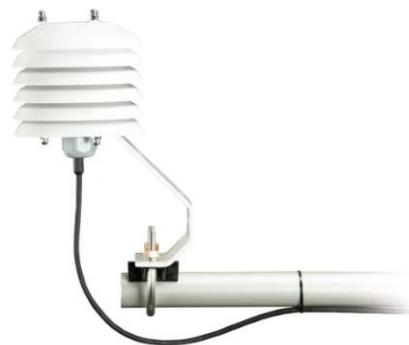
The RAD06 includes a 2 in. U-bolt with a plastic V-block. The U-bolt is placed in the holes on the side of the bracket for attachment to a mast or vertical pole. The U-bolt is placed in the holes on the bottom of the bracket for attachment to a cross-arm.
